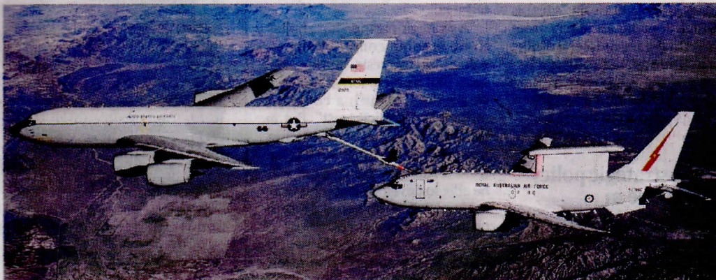
Taking on fuel mid-air greatly extends range and hours in the air
