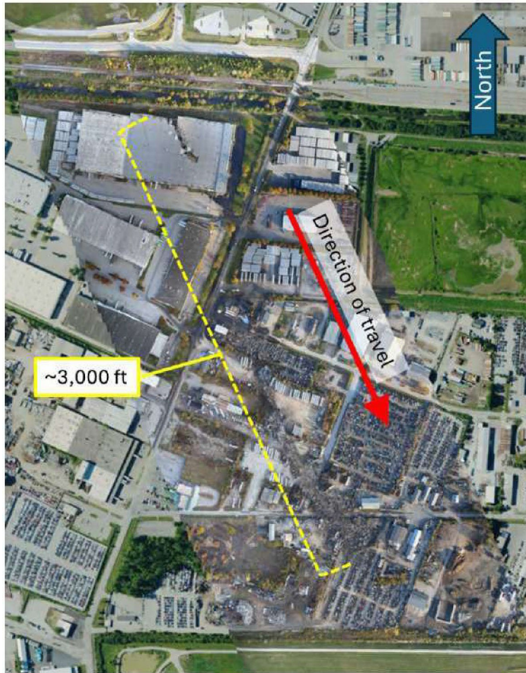
Figure 4. Accident site composite view created from aerial imaging overlaid on a Google Earth image. The upper end of the yellow-dashed bracket is the initial impact between the airplane landing gear and the UPS building roof.A
