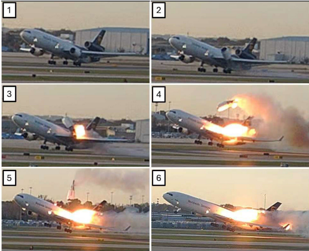
Figure 1. Still images from an airport surveillance video showing the left engine and left pylon separation from the left wing. (Source: UPS)
