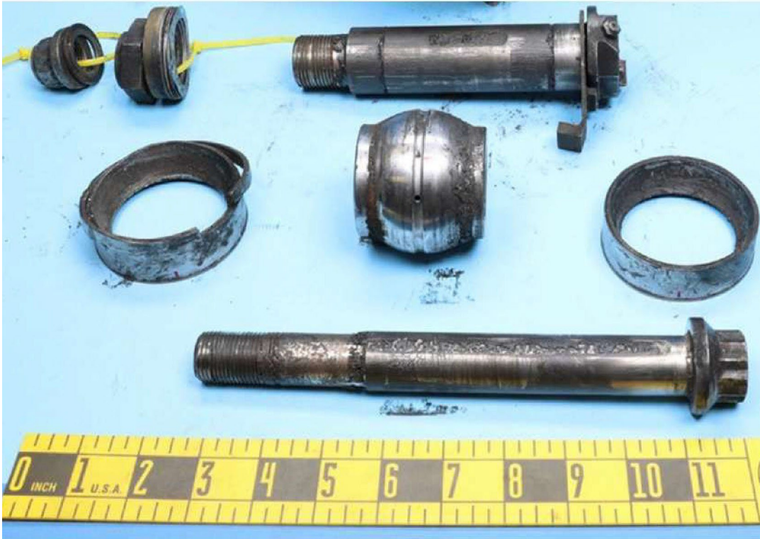
Figure 10. The spherical bearing and attachment hardware after removal from the left wing clevis.
